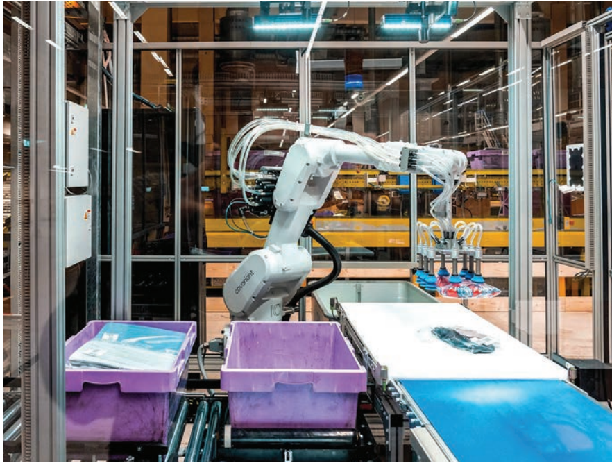
A Covariant robot demonstrates “induction”—the common warehouse task of placing objects on sorters or conveyors.
