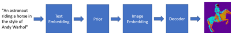
Figure 4-1. This shows the basic workflow for the DALL-E 2 model
